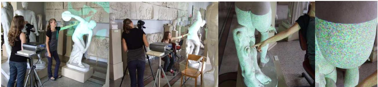
Figure 2: The acquisition process. The string helps to keep the camera at the same distance from the chosen surface point. The camera autofocus is switched off both for greater speed and accuracy.
