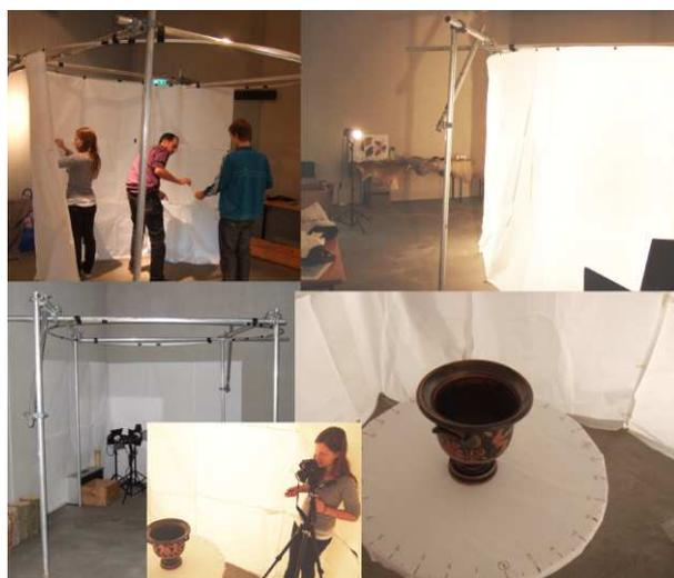
Figure 3: Artificial diffuse illumination. The paper cylinder is illuminated from outside to obtain as diffuse illumination as possible in its interior.
