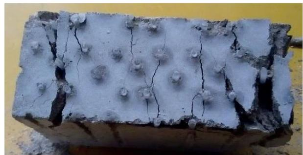
Figure 7: Image of LCTM failure (fiber diameter=1.5 mm).
