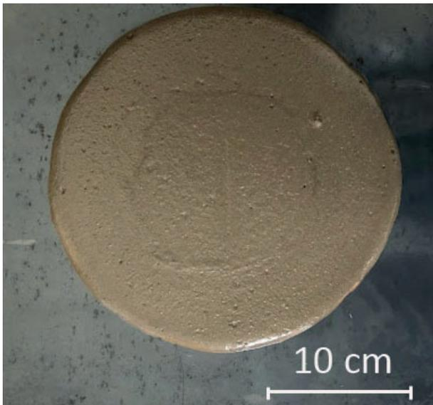
Figure 5: Image of mini-cone test.
