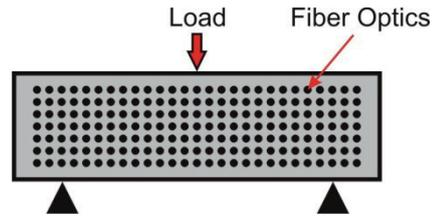
Figure 3: Schematic diagram of flexural test for LTCM.
