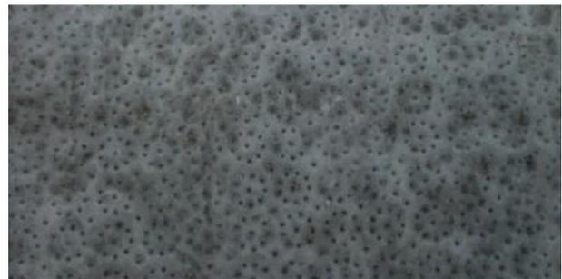
Figure 6: LCTM block surface (fiber diameter=0.75 mm).
