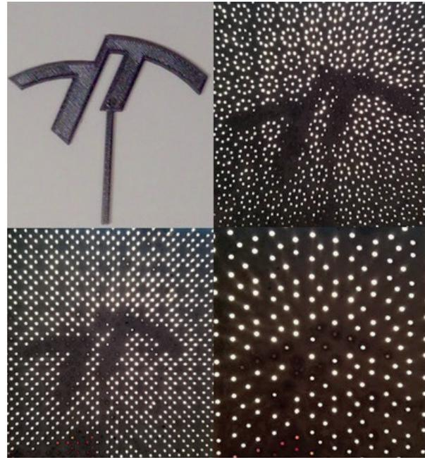
**Figure 9:** Effect of fiber diameter on shadow contour.
